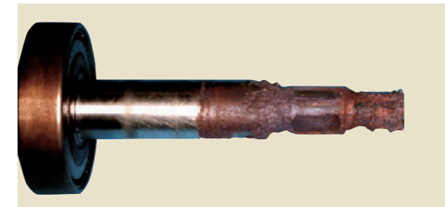
A cast 304 stainless steel impeller was mounted on 403 stainless steel shaft. (The shaft was heavily corroded.)
