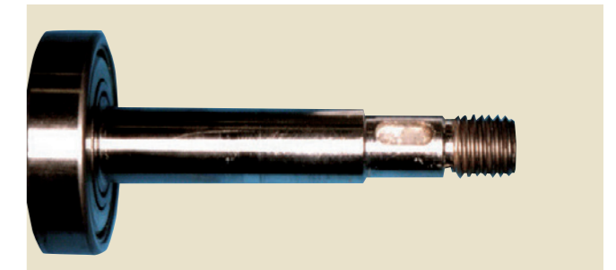
A seawater-resistant special cast iron impeller was mounted on 403 stainless steel shaft. (The shaft was protected against corrosion.)
