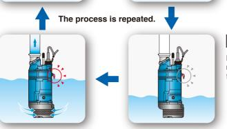
Pump stops in about one minute after the water level
