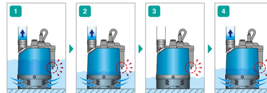
1 Pump continues to run while the electric probe remains submerged.
